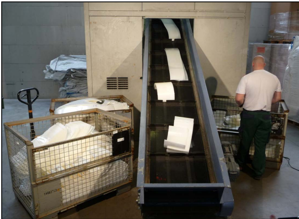
Material feeding towards the shredder.
