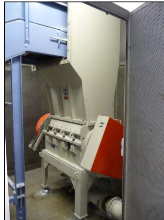
The material brought by the conveyor is hacked here and drawn out by a vacuum system (see tube).
