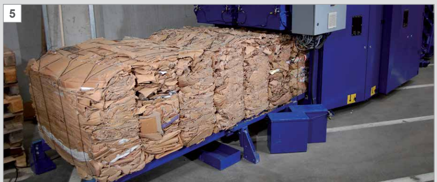
5 The export density bales can be stacked and are discharged fully automatically
