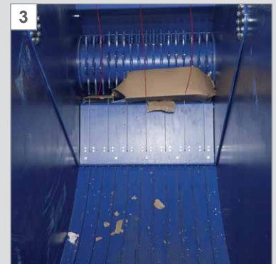
3 The strong rotor conveys the material into the pressing chamber.
