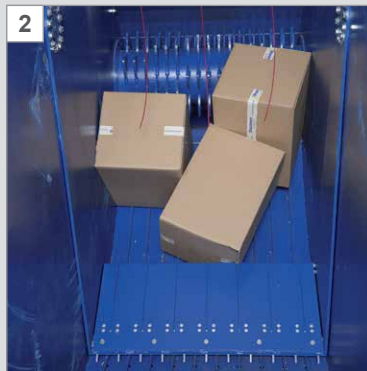
2 A swing device then pushes the material to the rotor.
