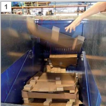
1 The material is thrown into the feed channel of the BaleTainer® without pre-shredding
